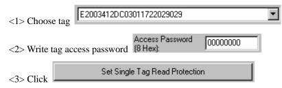
According to EPC number of the tag, setting read protection, make tag unable to be read and written by any order, even if query the tag, it is unable to get EPC number of the tag. Only NXP UCODE EPC G2X tags valid.
